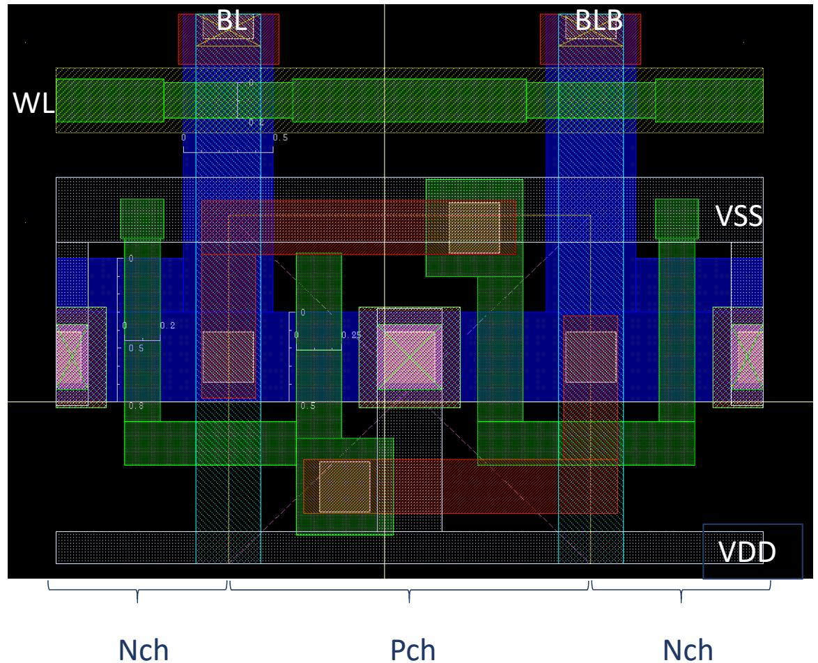
Cell Size :  $3.94\mu\text{m} \times 3.06\mu\text{m} = 12.06\mu\text{m}^2$
