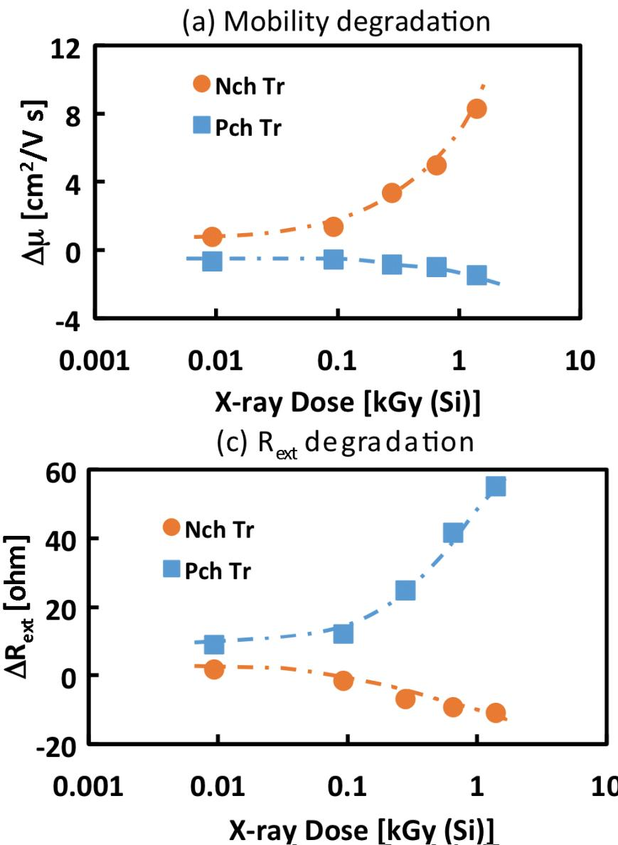
In PMOS, effective Gate Length become longer and Channel Resistance is increased with radiation.
