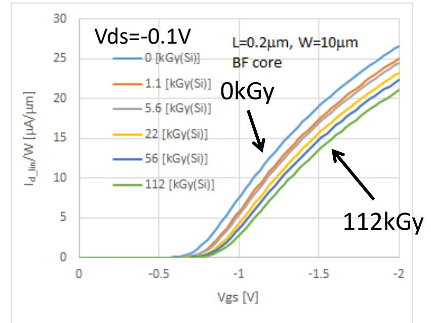
With increasing Implantation dose of PLDD region 6 times higher than present value, the degradation is reduced from 80% to 20% at 112 kGy(Si).
